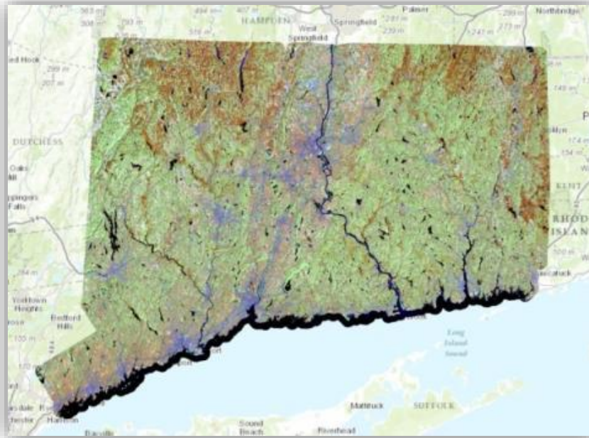
Landsat 8 Optical Land Imager (OLI) mosaic, acquired April 2014. Image is displayed showing near infrared reflectance as Red, middle infrared as Green, and Red as Blue.
